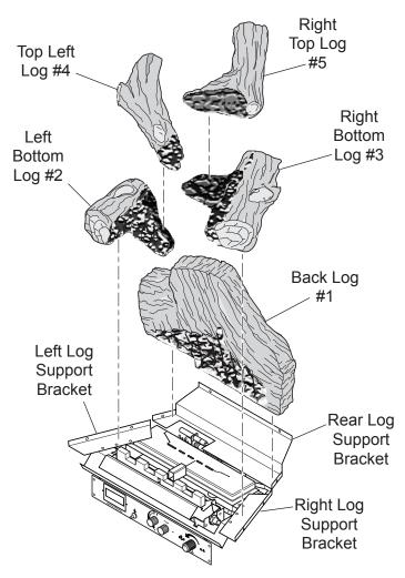
Figure 17 - Installing Logs to Grate
